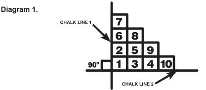
Slide tiles into position to prevent yarn from being trapped between the modules. Trapped yarn may adversely affect the overall appearance of the installation and can cause alignment problems.
