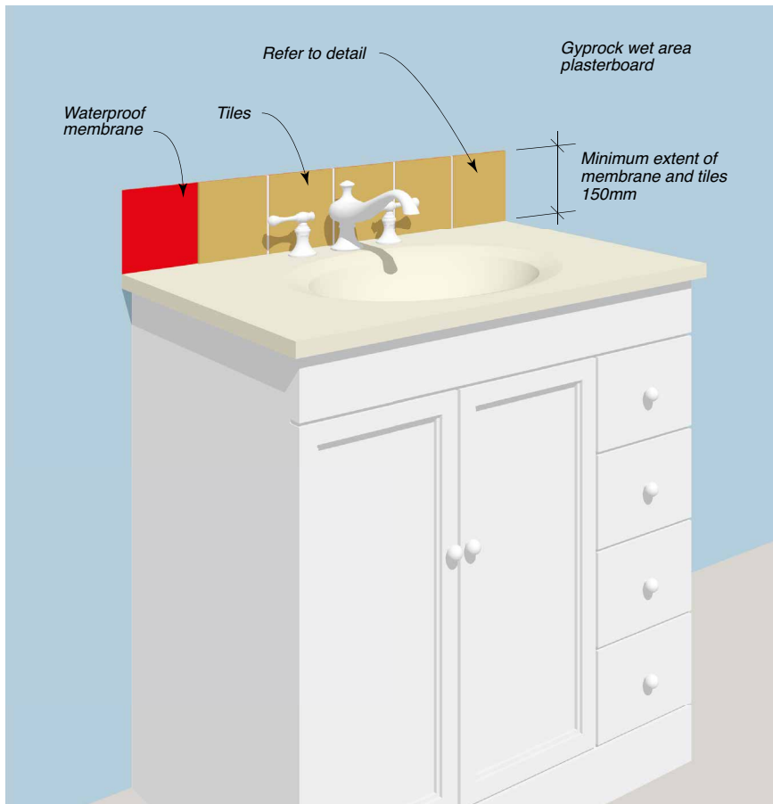
Figure 221: Typical Hand Basin – Membrane/Tiling Detail
