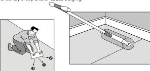
Joints do not require seaming by hot or cold welding.
