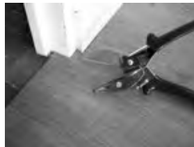
Moulting shears with mitre guide Gerflor : 0566 0001 Janser : 237 530 000 To cut around the feet of doorframes and in awkward places. Available from Gerflor
