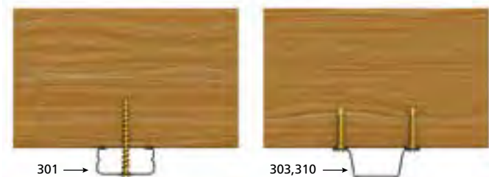
TRAFFICABLE FLOOR INSTALLATION DETAIL
