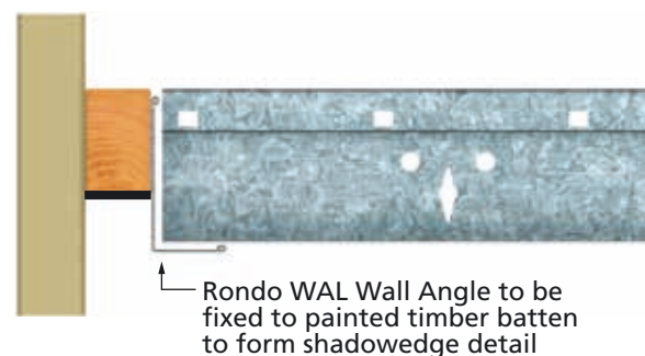
■ LONG LEG WALL ANGLE TYPICAL APPLICATION
